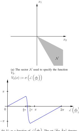
(b)  $V_2$  as a function of  $\angle \left(\frac{x}{|x|}\right)$ . The set  $\left[\frac{2}{3}\pi, \frac{5}{6}\pi\right]$  denotes the angles in the cone  $\mathcal{N}$ .
