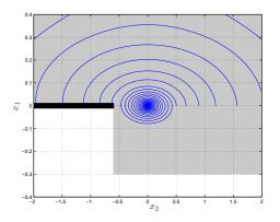
(b) After a finite number of jumps, the ball's trajectory remains in the flow set and asymptotically converges to A by only flowing.
