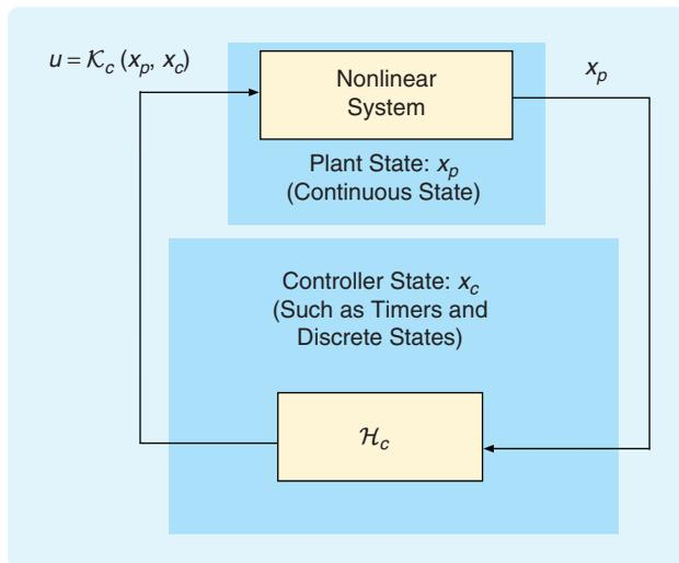
**FIGURE 6** Closed-loop system consisting of a continuous-time nonlinear system and a hybrid controller. The nonlinear system has state  $x_p$ , which is continuous, and input  $u$ . The hybrid controller has state  $x_c$ , which has continuous state variables, such as timer states, and discrete state variables, such as logic modes. The control input  $u = \kappa_c(x_p, x_c)$  to the nonlinear system is a function of the plant state  $x_p$  and the controller state  $x_c$ .
