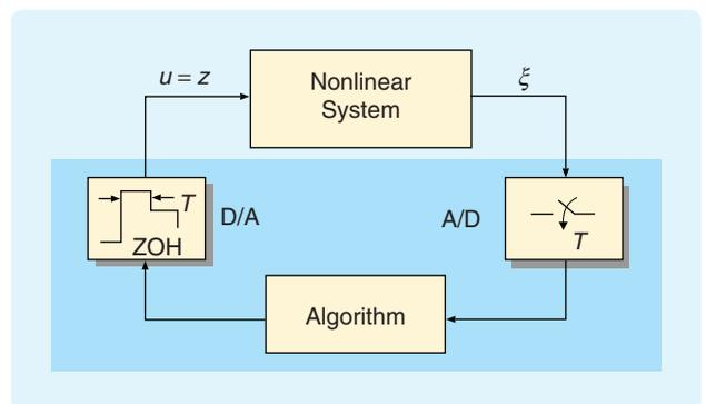
**FIGURE 5** Digital control of a continuous-time nonlinear system with sample-and-hold devices performing the analog-to-digital (A/D) and digital-to-analog (D/A) conversions. Samples of the state  $\xi$  of the plant and updates of the control law  $\kappa(\xi)$  computed by the algorithm are taken after each amount of time  $T$ . The controller state  $z$  stores the values of  $\kappa(\xi)$ .
