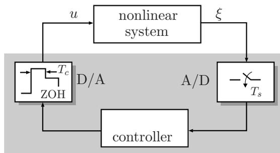
Figure 2: Sample-and-hold control of a nonlinear system.
