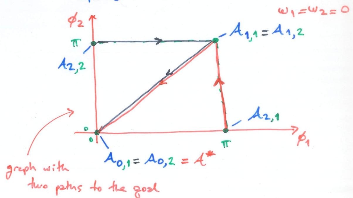
Throw-and-catch problem: Given  $A^*$  find local feedback controllers, open-loop controllers, and bootstrap controller such that the basin of attraction is the entire state space.
