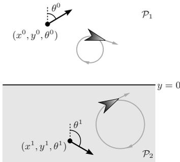
**Fig. 1.** Dubins vehicle on an heterogeneous terrain. The initial configuration is given by  $(x^0, y^0, \theta^0)$  and the final configuration by  $(x^1, y^1, \theta^1)$ . The forward velocity in patch  $\mathcal{P}_1$  is smaller than the forward velocity in patch  $\mathcal{P}_2$ .
