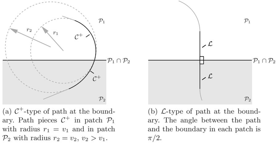
**Fig. 2.** Optimal paths nearby the boundary: paths of types  $C^+$  and  $\mathcal{L}$  satisfying the necessary conditions in Theorem 1.
