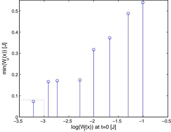
Fig. 5. Minimum energy (with respect to  $\mathcal{A}_r$ ) resulting from using  $\alpha_{r \rightarrow u}$ . The y-axis describes the minimum energy (with respect to  $\mathcal{A}_u$ ) resulting from the throw. Using  $c_u = 0.8$ , we confirmed that all initial pendubot positions with  $W_r(\mathbf{x}) < 10^{-3}$  can be caught by the controller  $\kappa_u$ .
