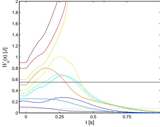
Fig. 4. The catch mode energy evolution for varying initial pendubot positions with near zero energy (with respect to  $\mathcal{A}_u$ ) using control law  $\kappa_u$ . All initial  $W_u(\mathbf{x})$  lower than 0.55 (solid black line) can be stabilized by the controller  $\kappa_u$ . The black dotted represents the  $c_u$  value that is used in the sublevel set  $L_{W_u}$ .
