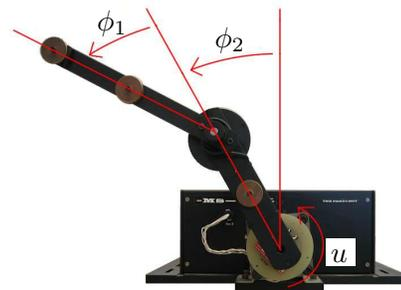
Fig. 1. The pendubot system: a two-link pendulum with torque actuation  $u$  in the first link.
