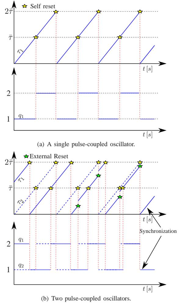
Fig. 1. (a) Trajectories  $(\tau_1, q_1)$  of a single pulse-coupled oscillator over two channels. (b) Trajectories  $(\tau_1, q_1)$  and  $(\tau_2, q_2)$  of two pulse-coupled oscillators over two channels.
